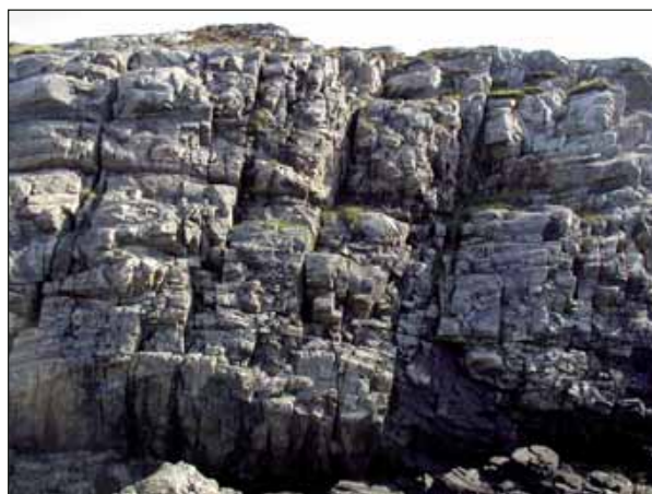
Figure 3: Long joints belonging to set 1 intersecting the rock masses. Some sub-horizontal foliation joints can also be seen. (Photo: Statoil / Norconsult)
