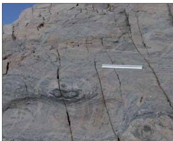
Figure 4: Joints of set 2. The ruler shown is 30 cm long. (Photo: Statoil / Norconsult)
