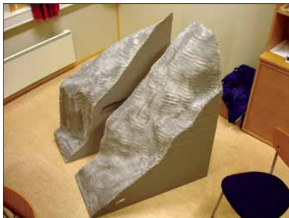
Figure 6 Model of the piercing area on a scale of 1:100
