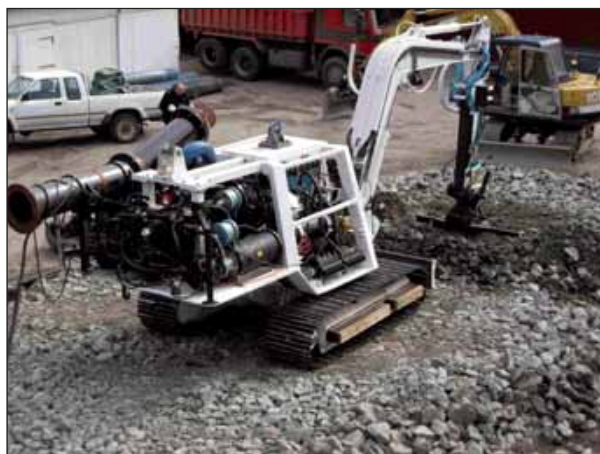
Figure 9 The SM03 tool carrier for the drilling unit.
