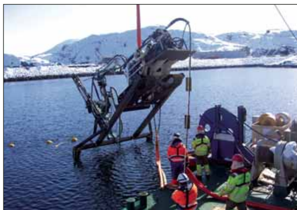
Figure 10 Lowering of SM03 with drilling unit
