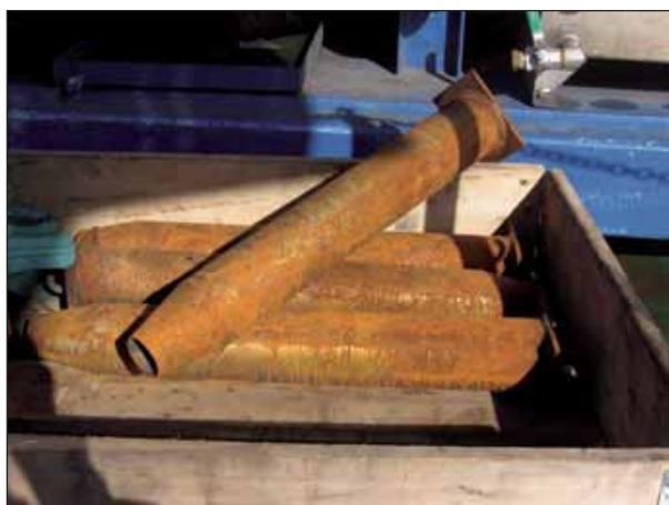
Figure 18 Steel cones for plugging boreholes that were drilled right through
