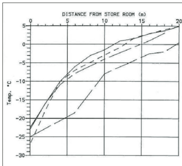
Figure 3: Temperature gradient in rock around a cold storage [Ref. 7]
