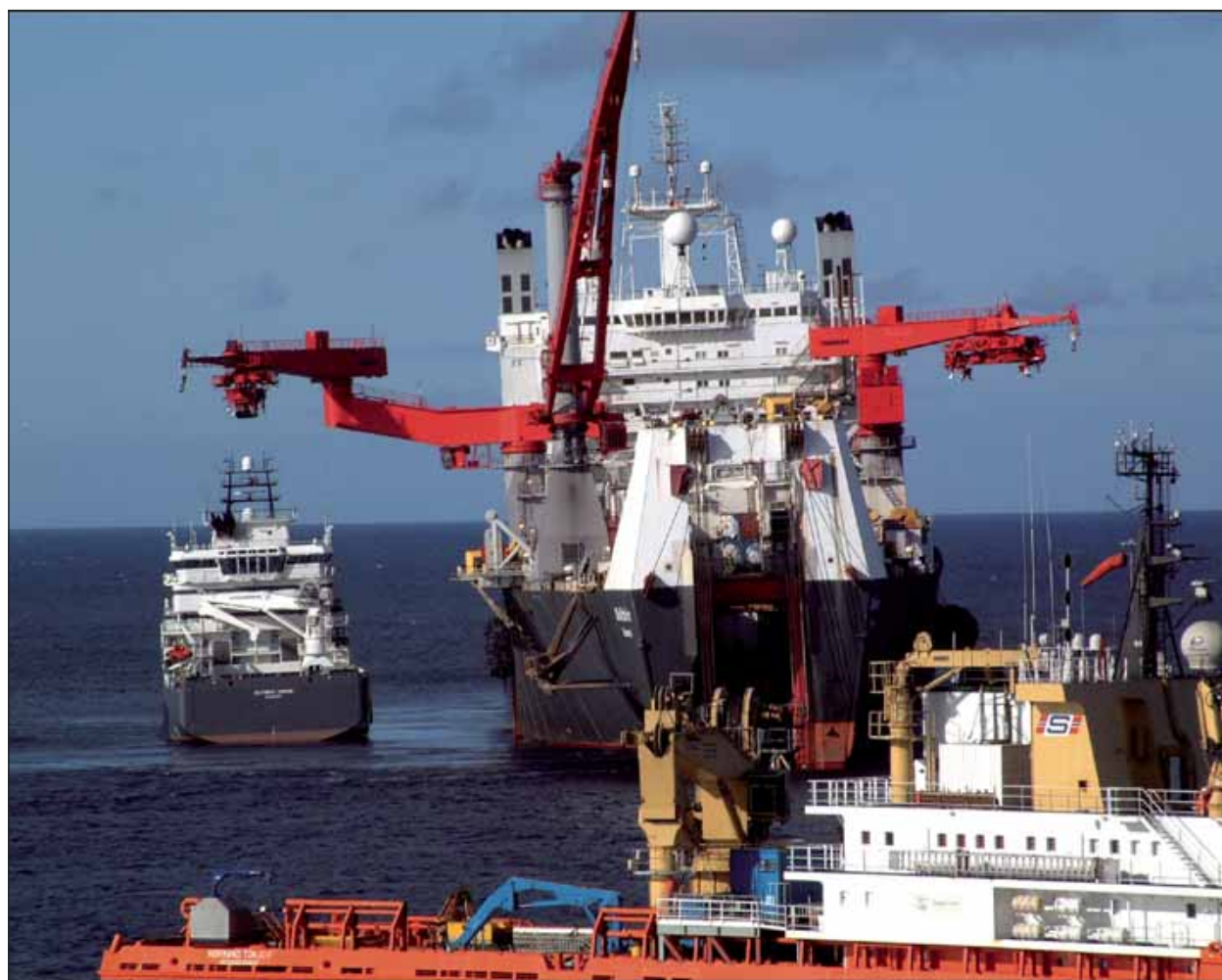
Figure 14: The lay-barge in position for pipeline pull-in (Photo: Norconsult)
