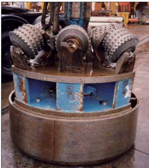
2. The 1600mm diameter reamer with stabilizer ring.
