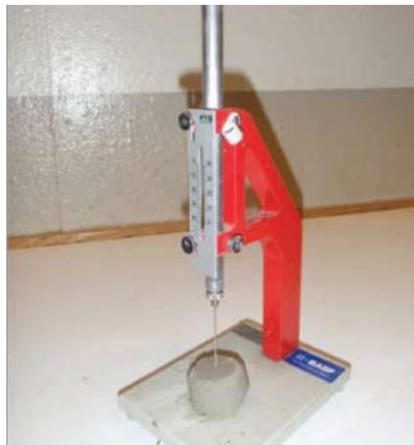
Figure 52. Vicat needle for testing setting.
