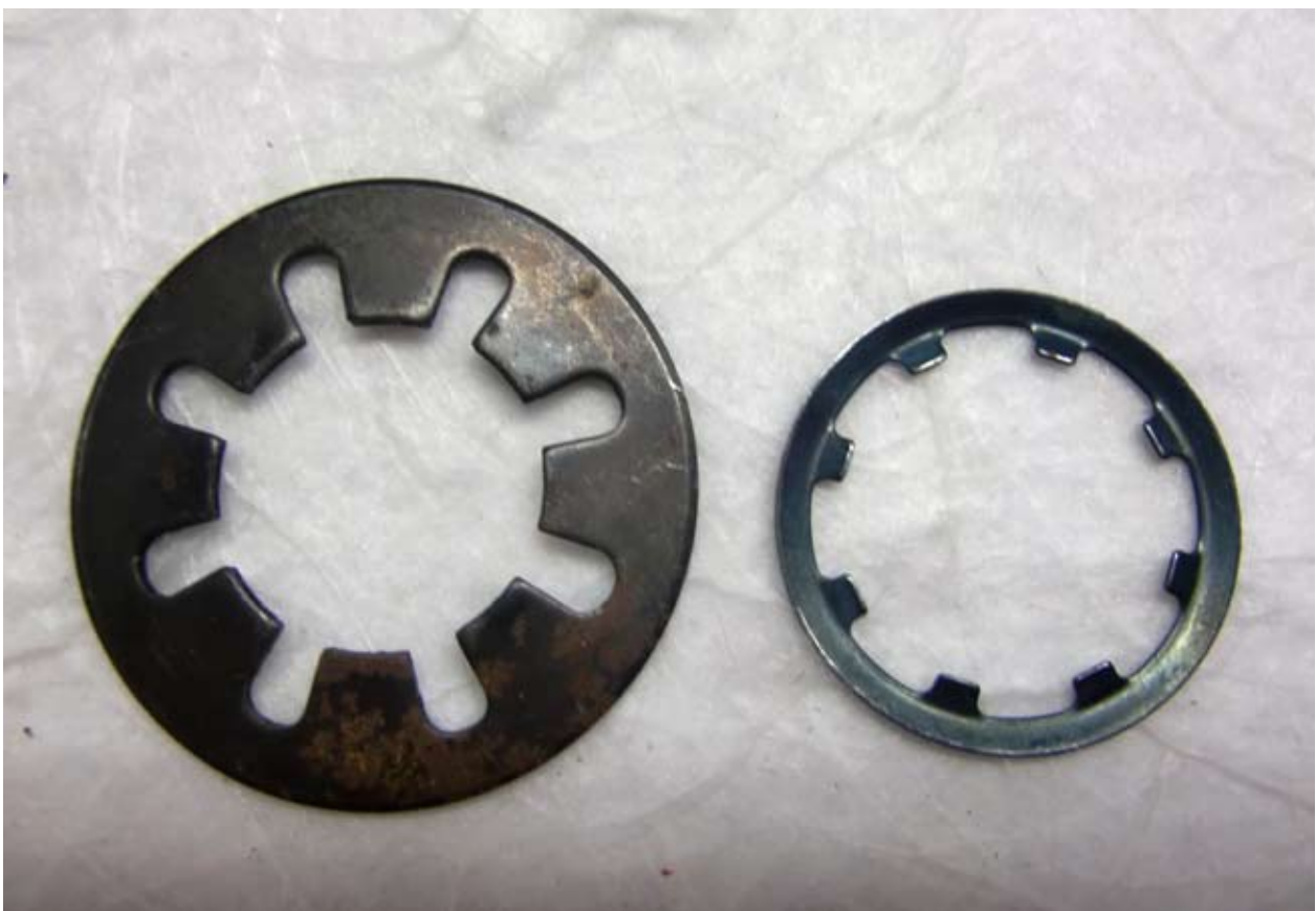
Figure 30. Certified lock bricks for Codan packers, 100 bars (left) and 60 bars (right) (photo: CODAN/Ivar F. Andersen)
