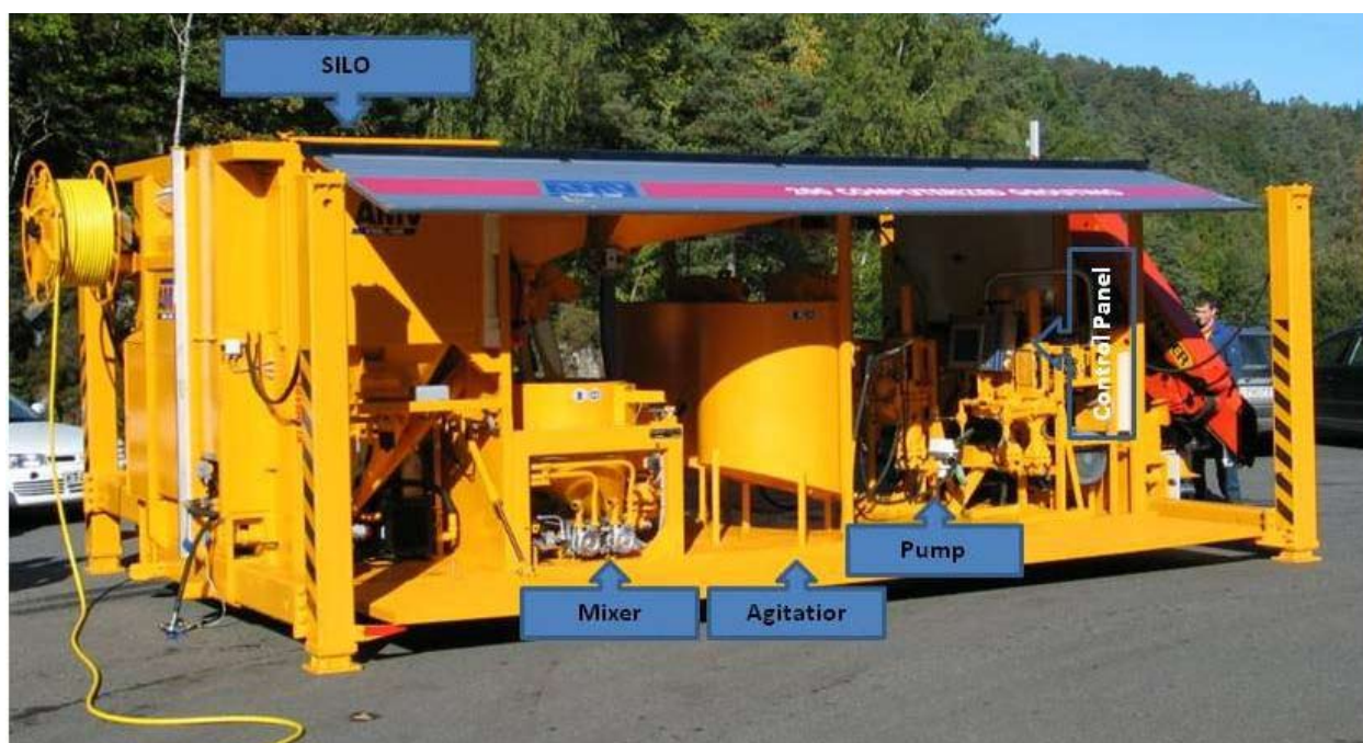
Figure 44. A modern grouting rig shall be complete, self-contained and prepared for easy transport to the next place of operation. Photo AMV.
