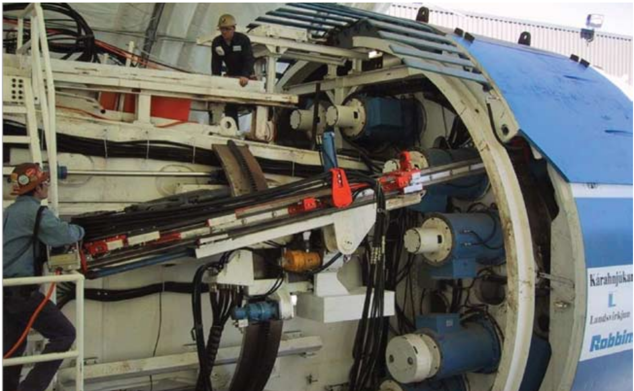
Figure 58. Probe drills on an open TBM
