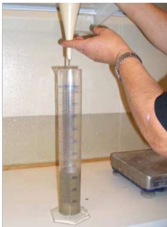
Figure 51. Checking w/c ratio using a Marsh cone
