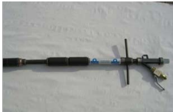
Figure 17. High-pressure packer with hydraulic tap and eye for chain on the left and a safety packer with extra tensioning on the packer body on the right (demo version with shortened rod).
