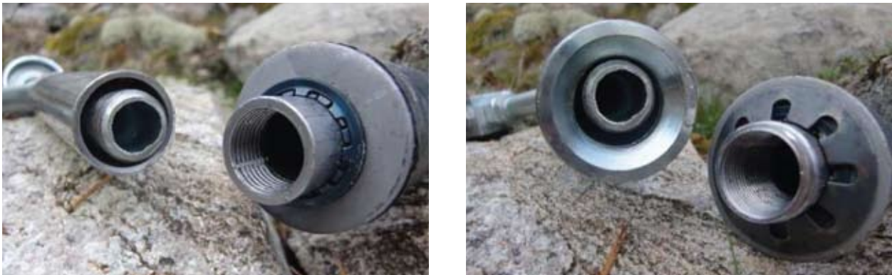
Figure 15. Packers with a seat for up to 60 bar on the left and up to 100 bar on the right.
