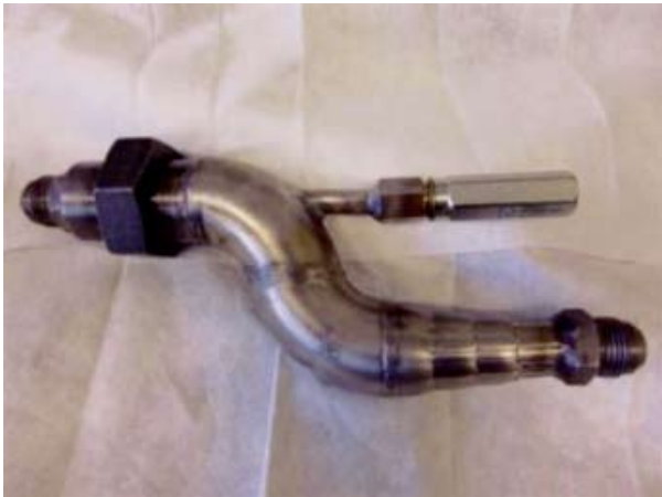
Figure 24. Injector for accelerator with non return valve (photo: CODAN/Ivar F. Andersen)
