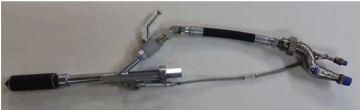
Figure 16. Complete rod with accelerator nozzle (demo version with shortened rod)
