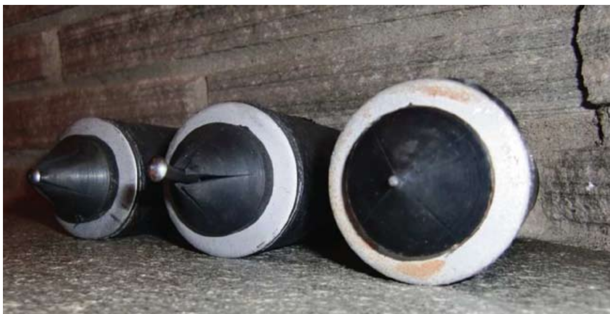
Figure 43. Packers that are open and allow water to pass through before they are grouted.
