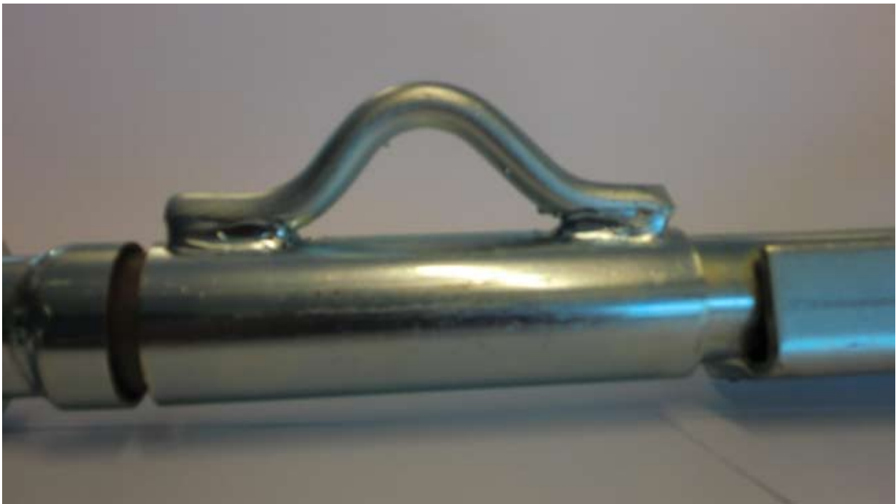
Figure 29. Safety chain fixing allow rotation of the grout pipe. Make it possible to leave the packer in the hole, and remove the pipe (photo: CODAN/Ivar F. Andersen)
