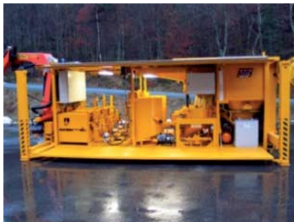
Figure 13. AMV automatic 3 line grout plant (Photo: AMV Group)
