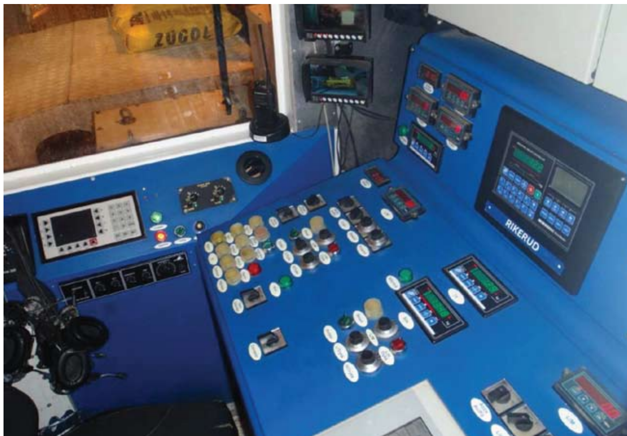
Figure 11. Example of a control panel on a modern grouting rig
