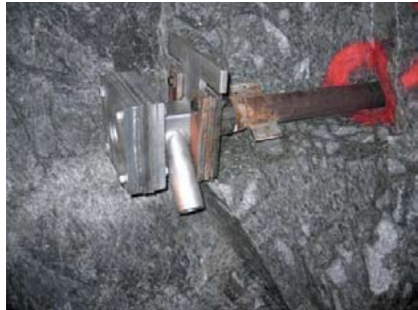
Figure 25. Sand pope with blow out preventer (photo: CODAN/Ivar F. Andersen)
