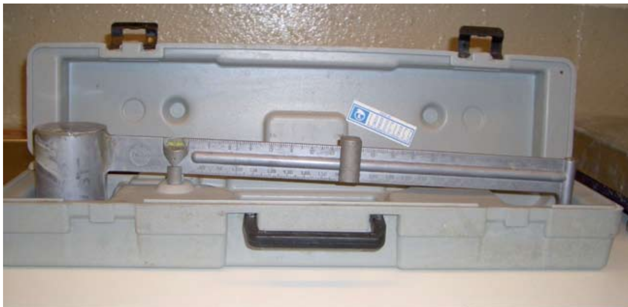
Figure 50. Specific gravity testing by mud balance scale (Photo: BASF)
