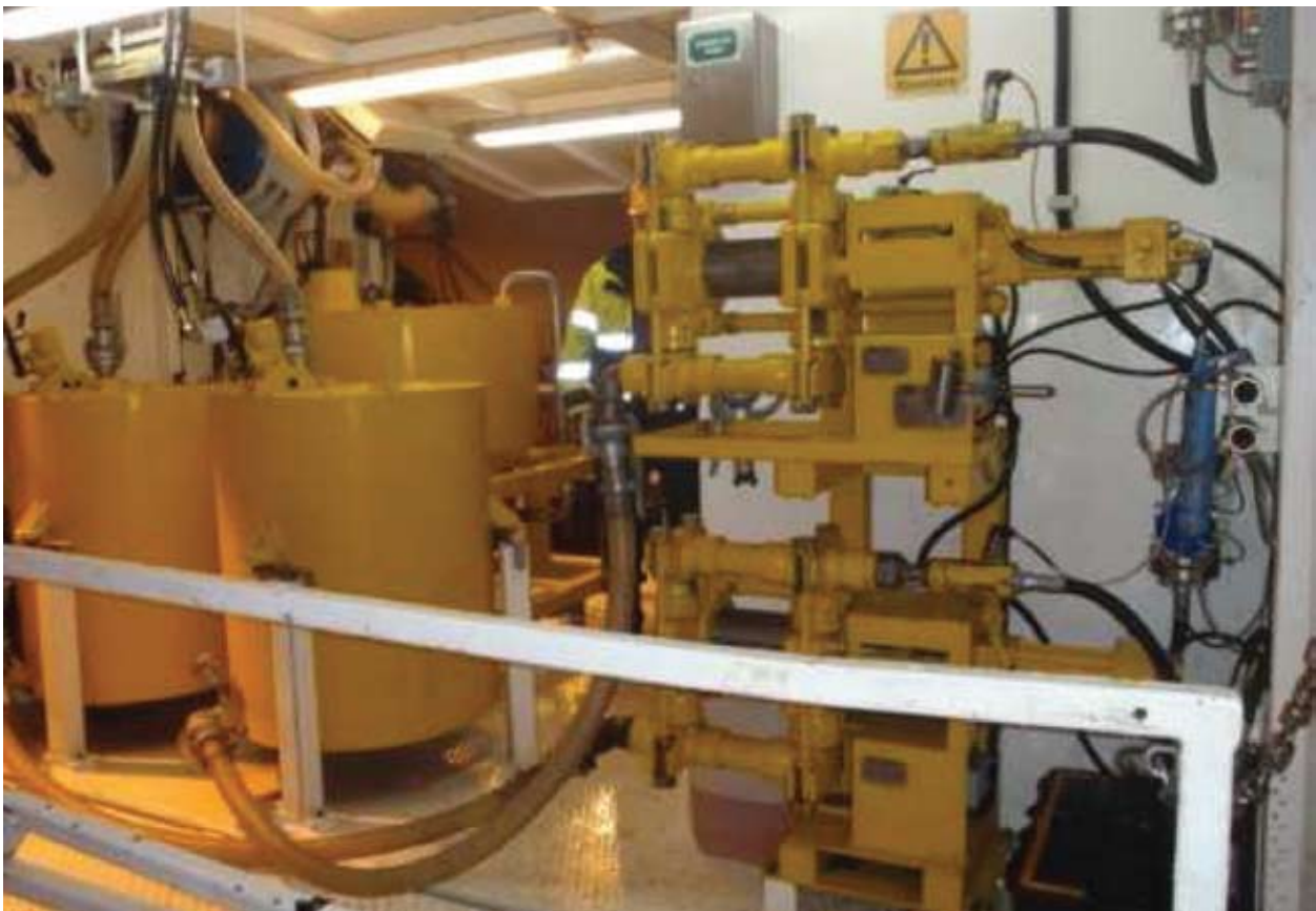
Figure 10. Example of equipment found on a modern grouting rig
