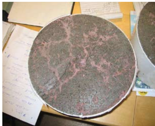
Figure 60. Test showing the spreading of polyurethane.
