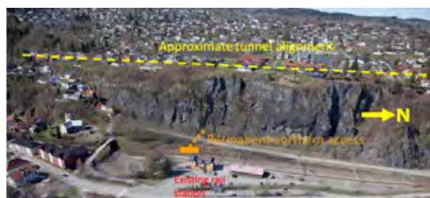
Figure 4: The up to 70 m high rock slope consist of volcanic rock. The cavern floor is at about the same elevation as the road just below the slope.
