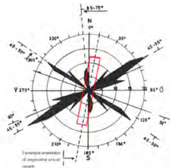
Figure 3: Favourable orientation of the longitudinal axis of a cavern or other underground opening in respect to the orientation of the dominating crack systems (Selmer-Olsen, R. And Broch, E. (1977)).
