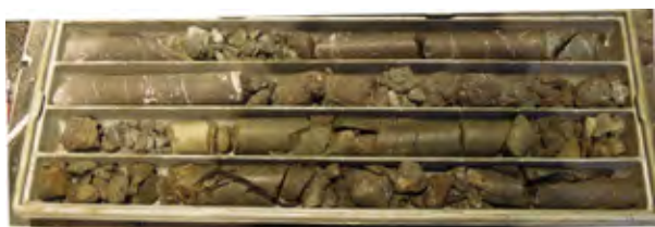
Figure 10: KH 11 drilled from the tunnel face through the major fault.
