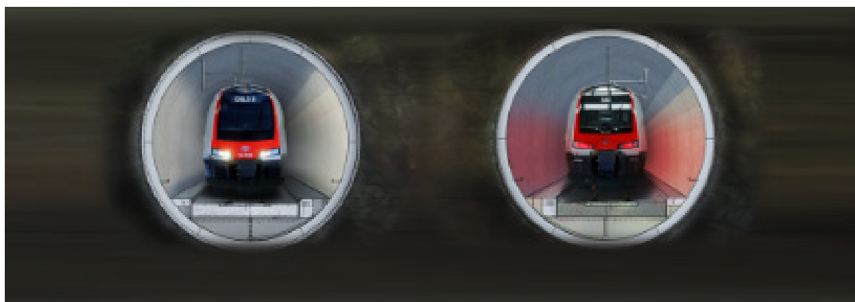
Figure 1-4 Two separate tubes with cross sections every 500 meters are chosen for the 20 km long tunnel, The Blix tunnel, at the Follo Line project.
