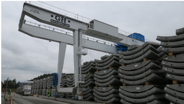
Figure 16-5: One of the storage areas with the gantry crane.
