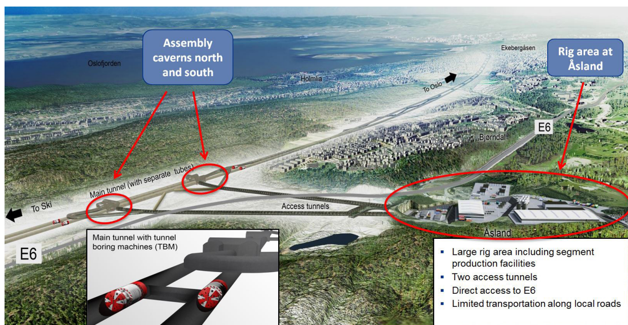
Figure 10-6: The TBMs were assembled in two centrally located large caverns.
