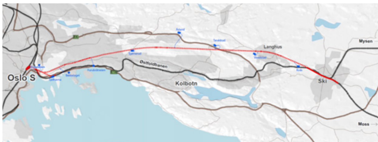
Figure 2-3: Excavation of the 18,5 km x 2 long tunnel by drill-and-blast required performance from seven access tunnels distributed along the tunnel in addition to the access tunnel required for excavation of the northern 1.5 km long tunnel.
