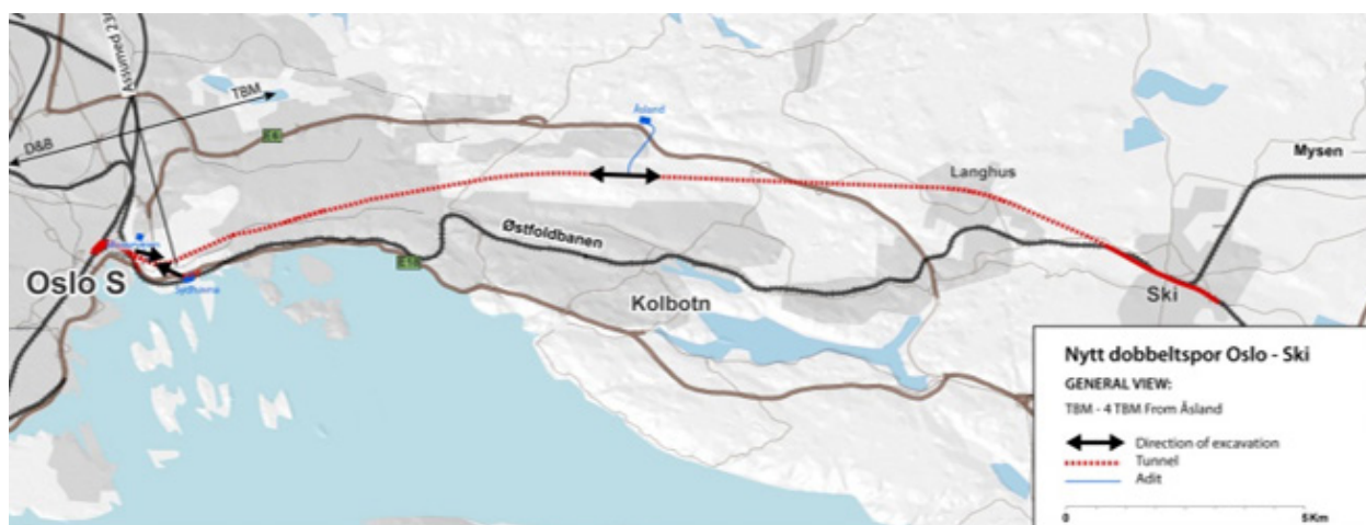
Figure 2-4: Excavation of the 18,5 km x 2 long tunnel by four TBMs operating from one centrally located rig area.
