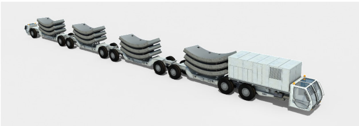
Figure 12-16: Segment MSV – 3D design.
