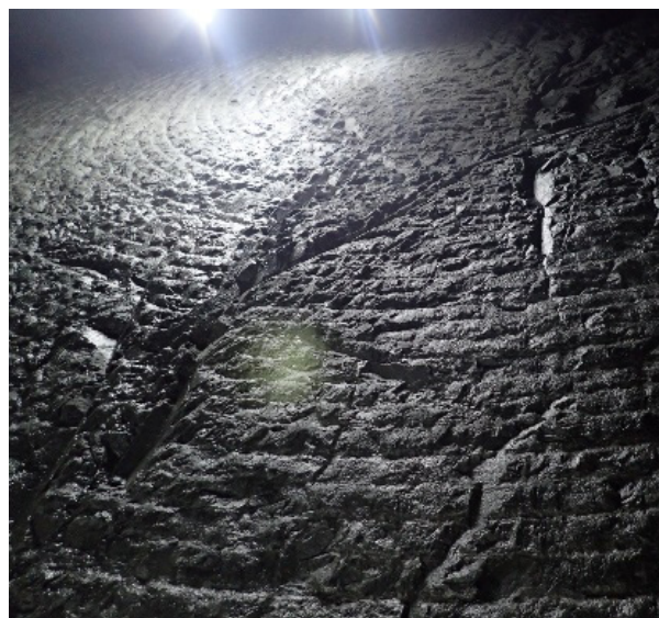
Figure 14-5: Fractures with different orientation identified at the face.
