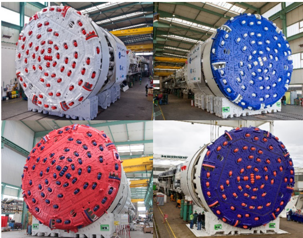
Figure 12-17: Upper row: TBM1 (S-980 Queen Euphemia) and TBM2 (S-981 Queen Ellisiv). Lower row: TBM3 (S-982 Anna from Kloppa) and TBM4 (S-983 Magda Flåtestad) after FAT at Herrenknecht Factory. Photo: Herrenknecht.
