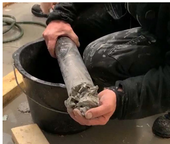
Figure 17-13: Left: Core sample of backfill grout, taken from the top of model B. Right: Core sample of backfill grout, drilled perpendicular through the concrete of model B.
