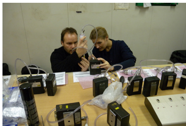
Figure 2: Calibration and set-up for the main exposure – rock dust.
