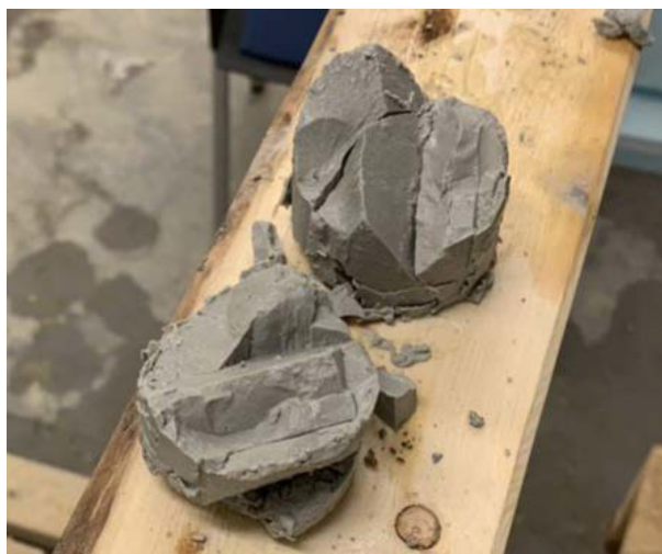
Figure 17-13: Left: Core sample of backfill grout, taken from the top of model B. Right: Core sample of backfill grout, drilled perpendicular through the concrete of model B.
