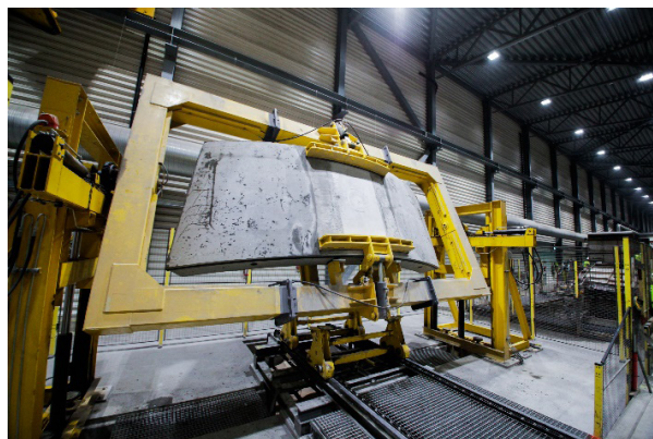
Figure 16-13: The carousel working line; Turing the segment around for "storage position".
