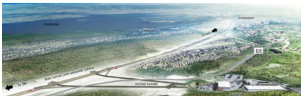
Figure 3-2: Adit tunnel system at Åsland.
