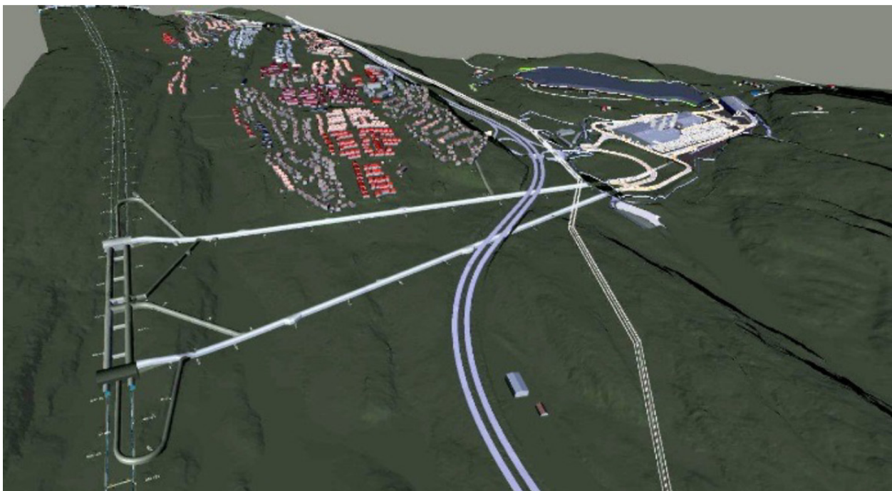
Figure 12-1: A 3D-model of the rig area located close to the main road (E6) and the access tunnel system with the caverns where the TBMs were assembled.
