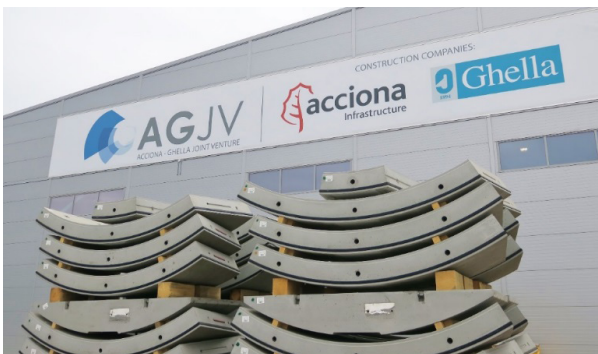
Figure 12-8: Two complete rings stored close to the precast factory.
