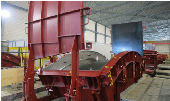
Figure 16-7: The carousel working line; Cleaned molds.
