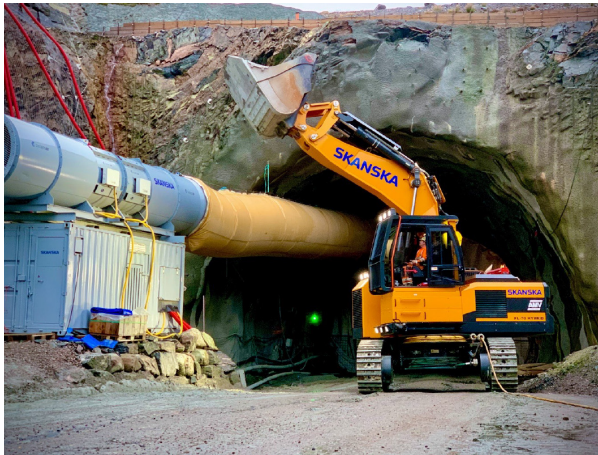
Figure 3.9.1. The new generation electric front loader, developed by AMW in cooperation with Skanska (Photo: Skanska).
