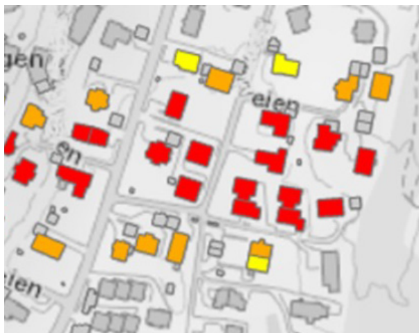
Figure 4.2.4. Section from ArcGIS view. Red marking high, orange medium and yellow low probability for noise above recommend limit values for tunneling works.
