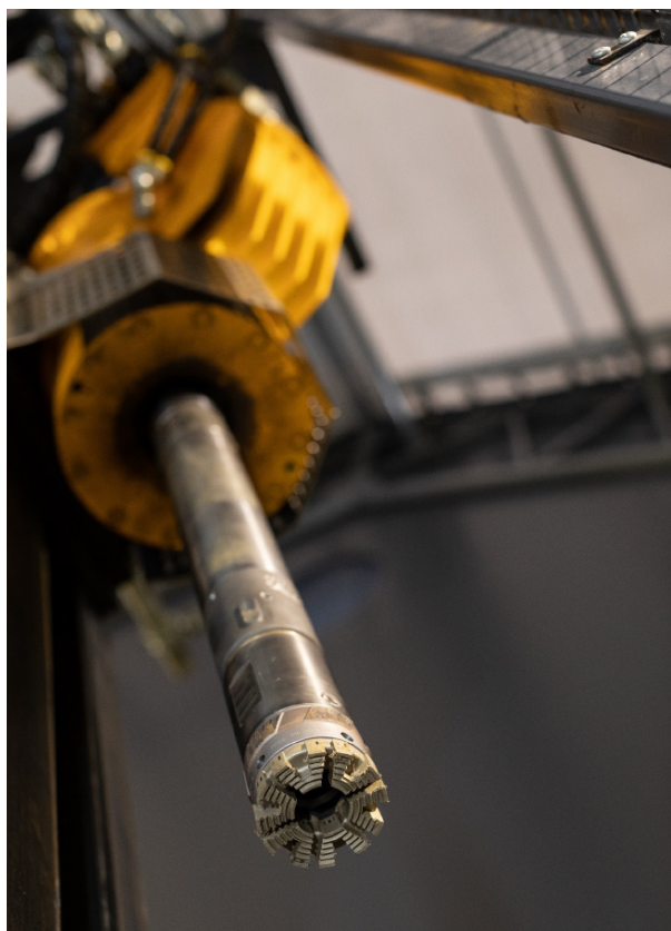
Figure 4.4.13. Detail picture of boring equipment (Photo: Devico).
