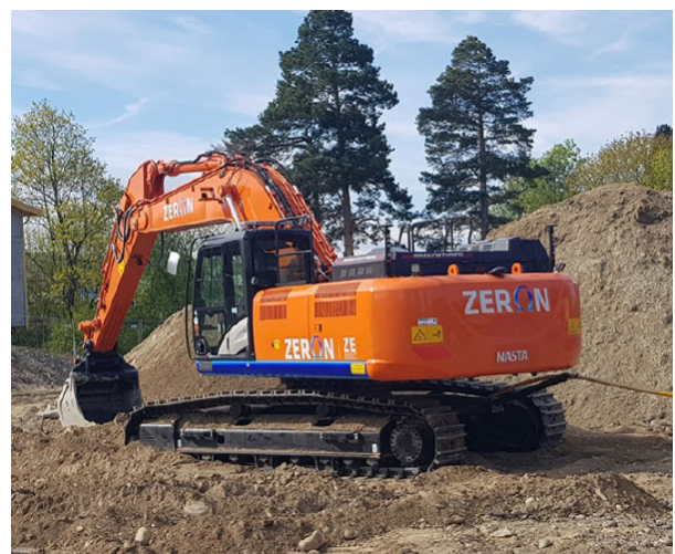
Figure 3.9.2. Zeron ZE350LC fully electric cable zero emission excavator.
