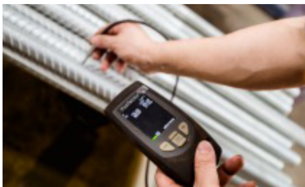
Figure 4.4.22. Control of coating thickness.
