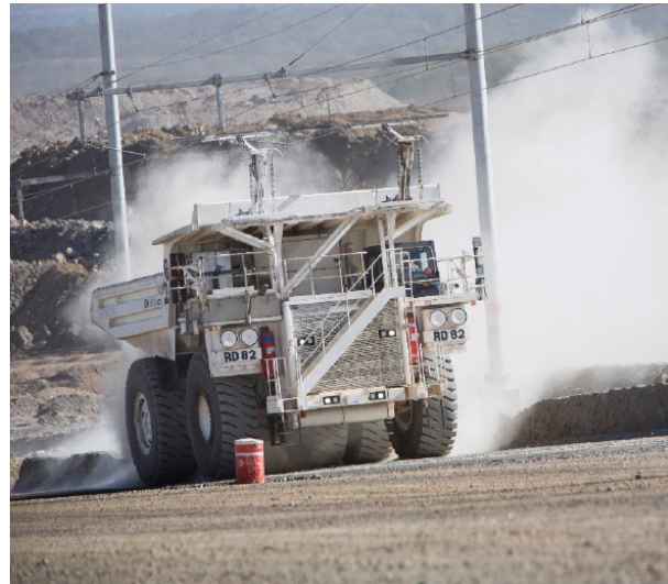
Figure 3.9.4. Hitachi 3500 AC truck soon available as battery and trolley (catenary) – zero emission.
