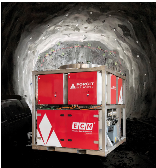
Figure 4.4.28. The new tunnel emulsion bulk charging unit EMC3.
