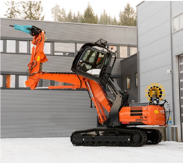
Figure 3.9.3. Hitachi ZX290LC custom made for de-scaling and securing of tunnels in combination with drill and blast – also available as electric.
