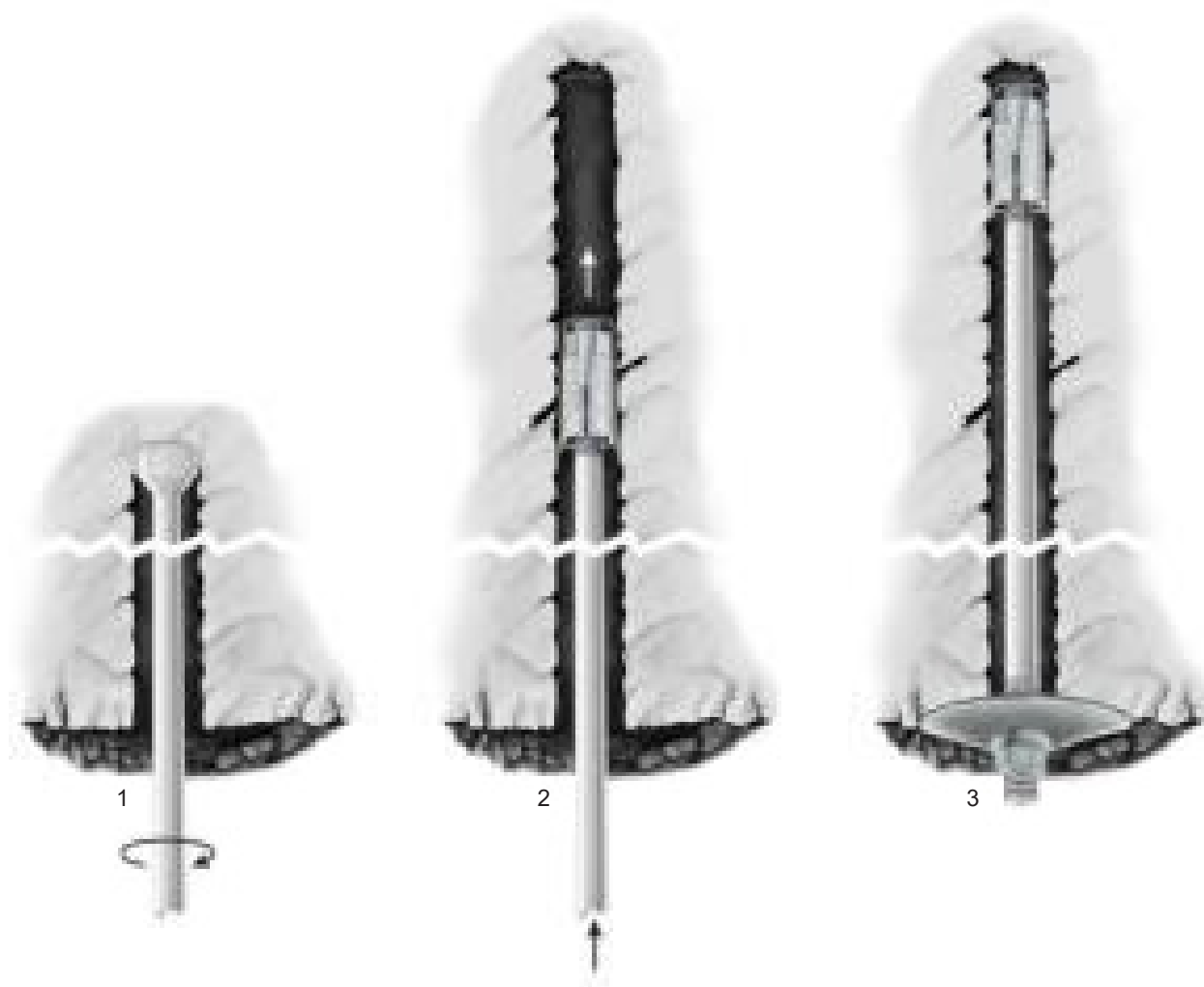
Figure 4.9 Installation of bolt using an expansion sleeve (end-anchored bolts).
