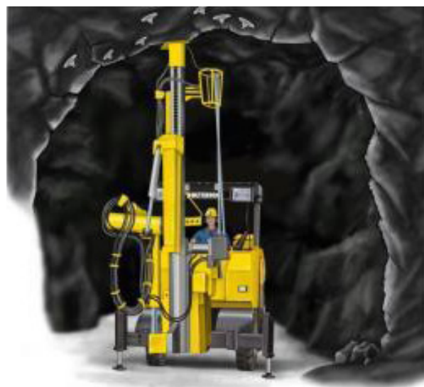
Figure 4.1 Fully mechanised bolting rig
