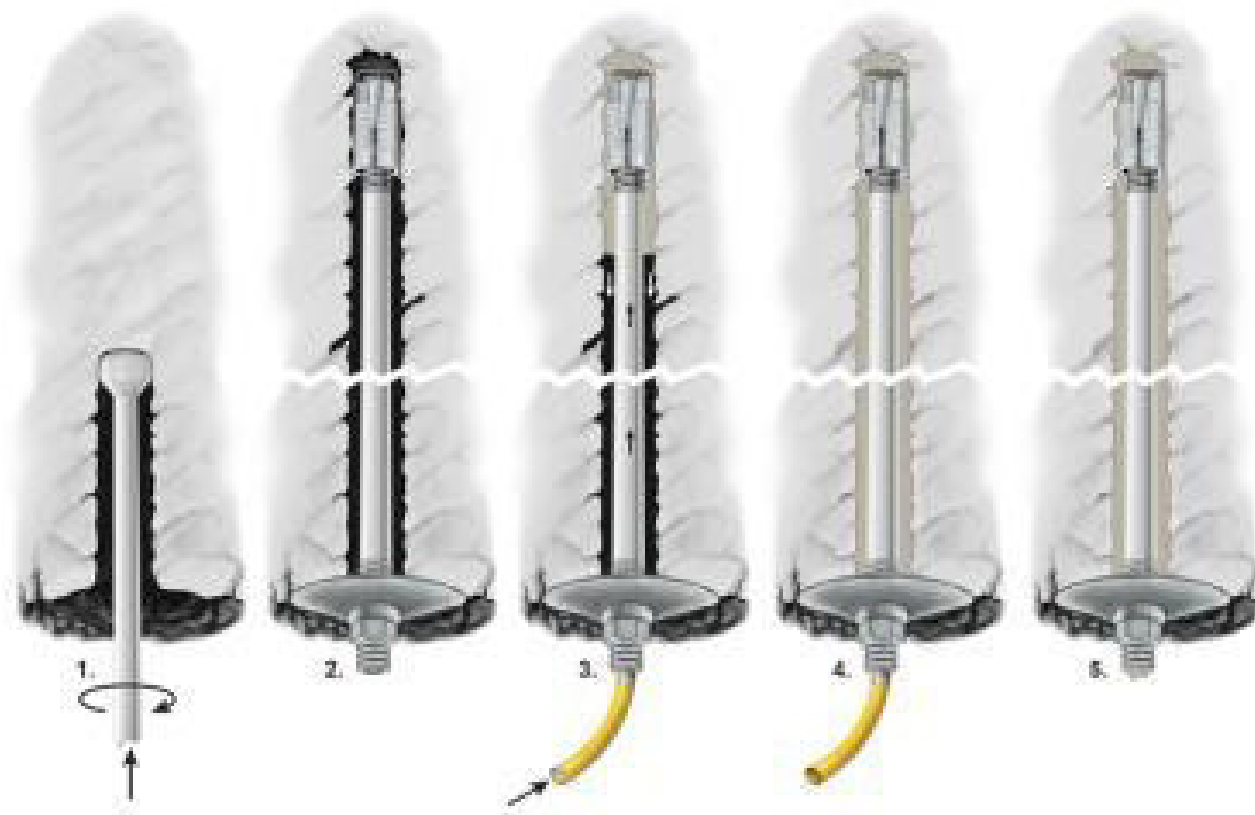
Figure 4.13 Installing a pipe bolt
